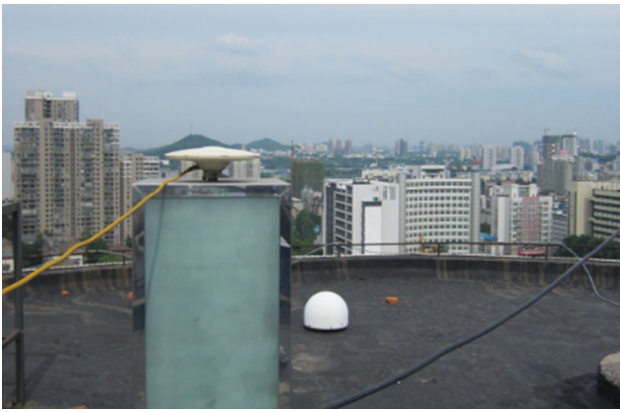
Fig. 2 Antenna connected to Trimble NetR9 receiver located on the rooftop of the GNSS Research Center at Wuhan University
