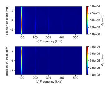
**Fig. 13.** FFTs of (a) crack aperture and (b) relative shear displacement change at the 15 points on the crack interface for the model with 30° inclined crack (a = 5.0e-5 mm) and subjected to the excitation wave with amplitude  $A_{dy} = 2.5e-4 \text{ mm}$ .
