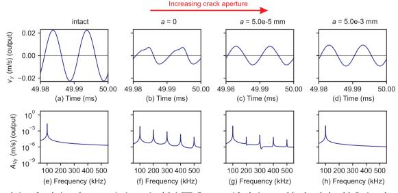
**Fig. 7.** Time evolutions of *y*-velocity at the sensor point (top row) and their FFTs (bottom row) for the intact model and cracked models (horizontal crack) with crack apertures a = 0 (closed crack), 5.0e-5 mm and 5.0e-3 mm, respectively. The models are subjected to compressive excitation wave with the amplitude  $A_{vy} = 3.1e-2$  m/s (i.e.  $\varepsilon_y = 1.0e-6$  and  $A_{dy} = 5.0e-5$  mm).
