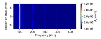
**Fig. 12.** FFTs of crack aperture change at the 15 positions on the crack interface for the model with horizontal crack (a = 5.0e-5 mm) and subjected to the excitation wave with amplitude  $A_{dy} = 2.5e-4 \text{ mm}$ .
