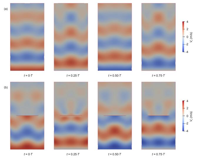
**Fig. 5.** Evolution of *y*-velocity within an excitation cycle *T* for (a) intact model and (b) model with a closed horizontal crack (i.e. a = 0) subjected to the excitation wave with the largest amplitude shown in Fig. 4 (i.e.  $A_{dy} = 5.0e-3$  mm and  $A_{vy} = 3.1$  m/s). The four time instances are respectively the beginning, first, second and third quarter of an excitation cycle.
