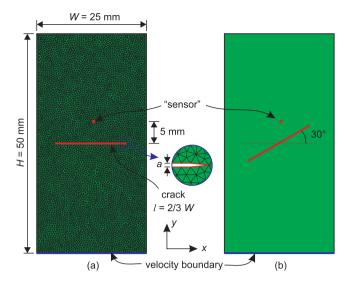
**Fig. 3.** Illustration of the FDEM model of a solid plate with a single crack: (a) horizontal crack located in the center of the plate and the corresponding mesh; (b) crack inclined 30° with respect to the horizontal direction and located in the plate center.
