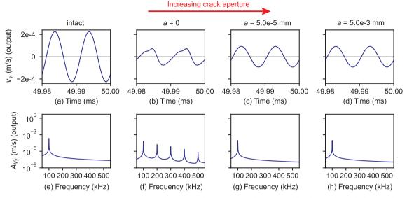
**Fig. 6.** Time evolutions of *y*-velocity at the sensor point (top row) and their FFTs (bottom row) for the intact model and cracked models (horizontal crack) with crack apertures a = 0 (closed crack), 5.0e-5 mm and 5.0e-3 mm, respectively. The models are subjected to compressive excitation wave with amplitudes  $A_{vy} = 3.1e-4$  m/s (i.e.  $\varepsilon_y = 1.0e-8$  and  $A_{dy} = 5.0e-7$  mm).
