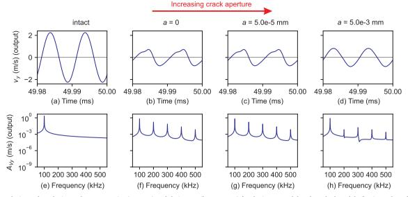
**Fig. 8.** Time evolutions of *y*-velocity at the sensor point (top row) and their FFTs (bottom row) for the intact model and cracked models (horizontal crack) with crack apertures a = 0 (closed crack), 5.0e-5 mm and 5.0e-3 mm, respectively. The models are subjected to compressive excitation wave with the amplitudes  $A_{vy} = 3.1$  m/s (i.e.  $\varepsilon_y = 1.0e-4$  and  $A_{dy} = 5.0e-3$  mm).
