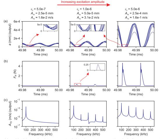
**Fig. 10.** Response of the model with horizontal crack (a = 5.0e-5 mm) and subjected to excitation waves with amplitude of  $A_{dy} = 2.5e-5 \text{ mm}$ , 5.0e-5 mm and 2.5e-4 mm, respectively: (a) time evolution of aperture a at the 15 positions on the crack interface; (b) time evolution of overall normal contact force  $F_N$  between crack surfaces; (c) FFT of *y*-velocity at the sensor point. The insets give a zoom-in of the results at specific time range.
