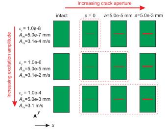
**Fig. 4.** FDEM models with increasing crack aperture and subjected to excitation waves with increasing amplitudes are created to investigate the relationship between crack aperture and nonlinear phenomena generation. Note the intact models are used for comparison purposes. The models located in the dashed rectangles are expected to generate nonlinear phenomena because of their potential of clapping between crack surfaces.
