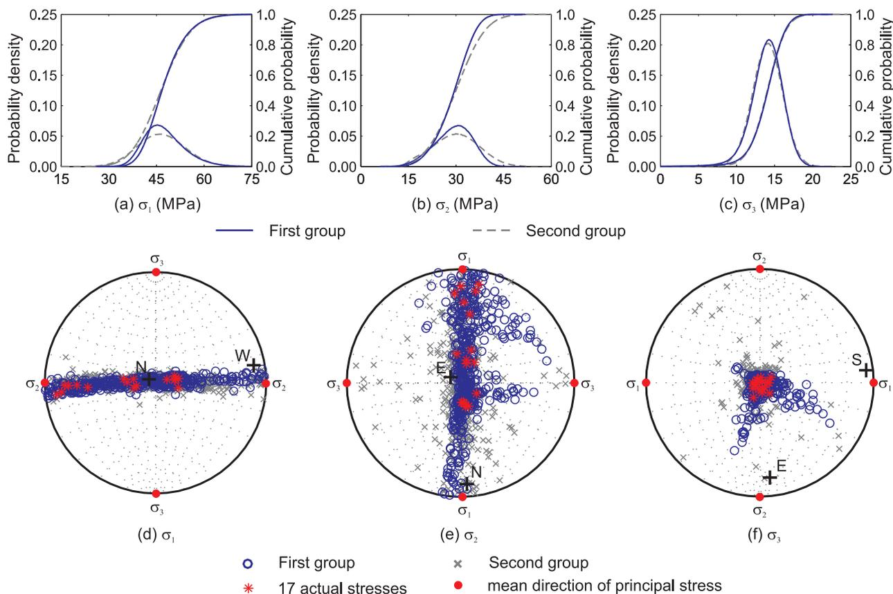
**Fig. 4.** Distributions of principal stress magnitudes and hemispherical projections of principal stress orientations of two groups of random tensors (for clarity the projections show a random selection of only 500 generated tensors, and have been rotated to place the mean at the centre of the projection and the other two principal stress directions at the N-S and E-W positions) (after Gao & Harrison<sup>38</sup>).
