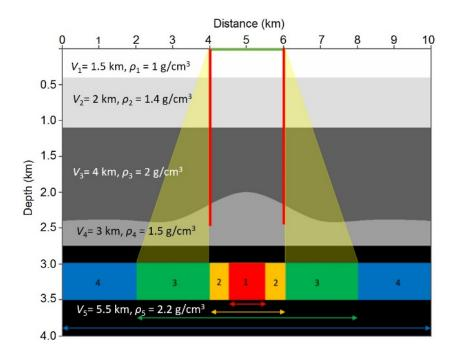
**Figure 13.** The geological model used in this study. Noise boundary 1 (red) laterally extends from 4500 to 5500 m; noise boundary 2 (yellow) extends from 3000 to 6000 m; noise boundary 3 (green) extends from 2000 to 8000 m; and noise boundary 4 has the same lateral extent as the model. The yellow triangles show the ideal range for the surface geometry that is between  $0^{\circ}$  and  $33^{\circ}$  (between noise boundaries 2 and 3).
