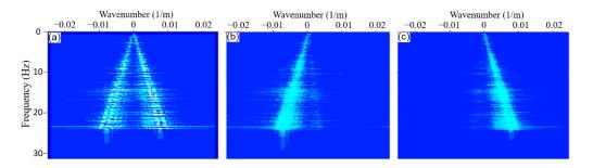
**Figure 10.** Separation of the downgoing wavefield and the upgoing wavefield; (**a**) before frequencywavenumber filtering, (**b**) the downgoing wavefield positioned in the positive quadrant, and (**c**) the upgoing wavefield positioned in the negative quadrant.
