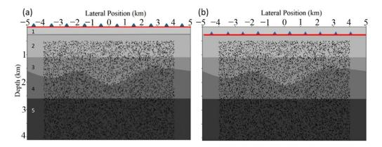
**Figure 3.** The geological mode used in this study. The red line with blue triangles shows the location of receivers. The dots show 1000 noise sources locations from deeper layers. In ( $\mathbf{a}$ , $\mathbf{b}$ ) the red line shows the acquisition line above and below the weathered layer, respectively. The sources are randomly distributed below the depth 500 m and within the offset -4000 to 4000 m.
