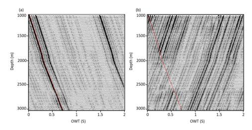
**Figure 11.** The separated (**a**) downgoing and (**b**) upgoing wavefield. The red line shows the P-wave downgoing primary trend in Figure 9.
