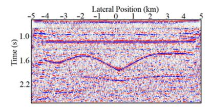
**Figure 6.** Stacked buried-geophone section after applying predictive and spiking deconvolution, and Radon transform filter. We note that the Radon transform significantly removes the surface multiples that remained in Figure 5 indicated by the arrows.
