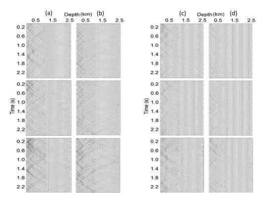
**Figure 14.** Virtual shot gathers created from the crosswell survey for noise generated within boundaries 1, 2, 3 and 4, in columns (**a**–**d**), respectively. The top images represent base surveys, the middle images repeat surveys, and the bottom images the difference between base and repeat surveys.
