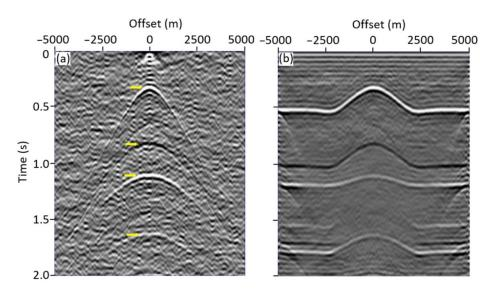
**Figure 8.** (a) A virtual shot gather retrieved at position of receiver 101 and (b) the final stacked section retrieved from the surface acquisition scheme. The yellow arrows correspond to the reflections from four interface in Figure 7.
