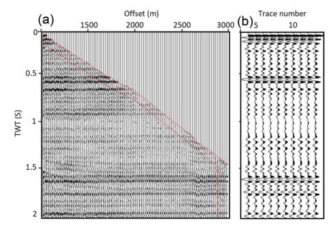
**Figure 12.** (a) The flattened upgoing wavefield. The red narrow corridor corresponds to the outside corridor stack, containing 10 traces. The receivers on the VSP in the borehole are starting from 1000 m to 3000 m. (b) The corridor stack that consists of 10 traces corresponding to the red narrow corridor.
