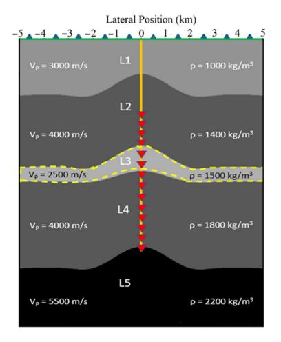
**Figure 7.** An acoustic velocity model with anticlines that are combined surface seismic and zero-offset VSP geometry. Blue triangles correspond to 201 geophones that are placed on the free surface. L3 (covered by yellow-dashed area) corresponds to the coal layer. The red triangles in the vertical direction (101 geophones) show the array of the geophones for VSP acquisition.
