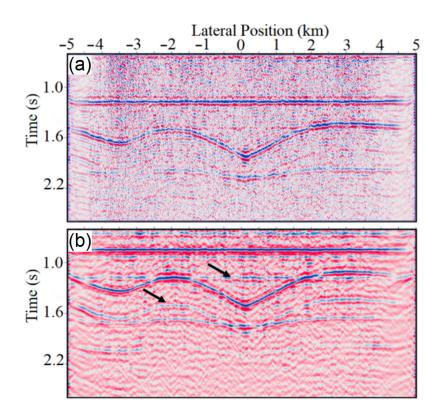
**Figure 5.** Stacked seismic section using geophones on (a) free surface and (b) beneath the attenuating weathered layer (Q = 30) corresponding to the geological model in Figure 3a,b. Arrows show downgoing surface multiples with the late arrival time of around 0.33 s comparing to their primary reflections.
