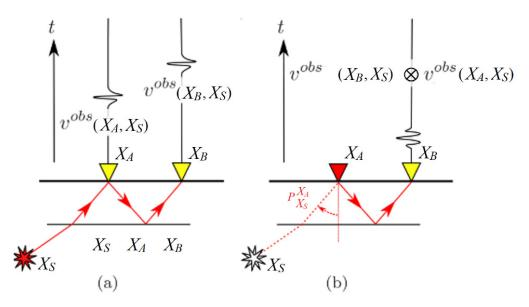
**Figure 1.** The fundamental principle of reflected-wave interferometry. (a) The subsurface source is emitted a signal from underground to the surface and is recorded by two geophones. The second geophone receives the reflected signal by an underground scatterer. (b) The cross-correlation cancels the common path from the source  $X_B$  to the first receiver  $X_0$ , as if a source were located at receiver  $X_0$ . The symbol  $\otimes$  denotes cross-correlation.
